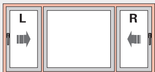
Diagram K 2 sliding sashes (L and R) 1 fixed glazing
